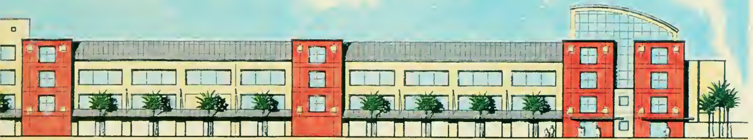
North Elevation. Carnival Cruise Line's Piers 6 and 7 expansion plan, San Juan. Ground floor with entry at one end, customs at the other, three baggage sections in between. Daylit third/fourth floor houses large waiting area with security and check-in facilities below, small boarding hall above.
